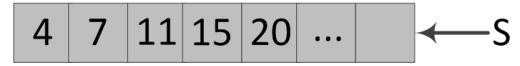
Figure 11: Result of prefix sum operation on T , based on spatial subdivision in Fig. 8. Each entry represents an object's offset based on the number of bins it touches.
