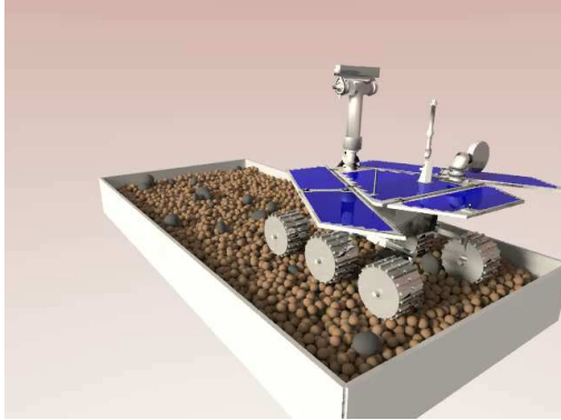
Figure 1: Chrono::Engine [1] simulation of a complex, rigid multi-body mechanism with contacts and joints.
